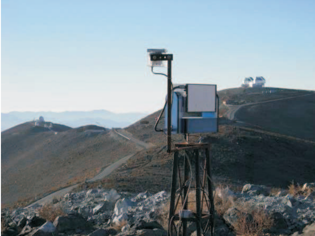
Figure 4. An IRMA unit installed at the Las Campanas Observatory.
